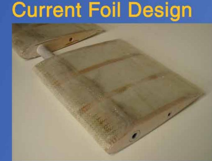
The design above shows the method of construction used for the previous year's foils. The method proved very labour intensive and produced a heavy final product. This years work is looking to generate a far more lightweight and versatile design that can be applied to a batch production system of manufacturing.
